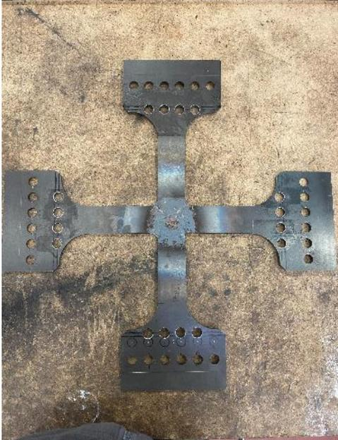
12.5kN Transient Heat to Failure
