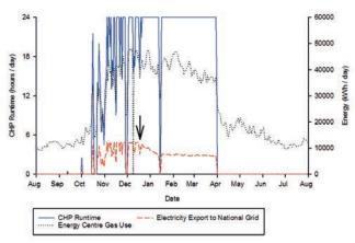
Figure 1.3. The electricity generation (red line) and the runtime (blue line) of the CHP. The arrow shows the event that led to the decrease in electricity generation.
