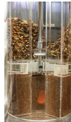
Figure 2 – Ultrasound Sensor with Rotating Mirror to Scan Ground Conditions from Inside of Pipes
