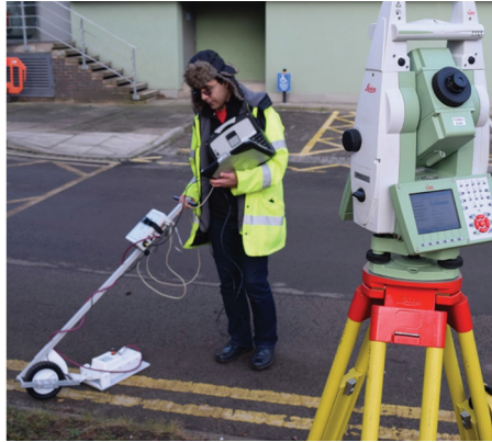
Figure 5 – Obtaining a 1.5 GHz GPS Survey of the Same Area
